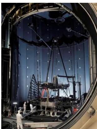
SESL Chamber A with JWST Pathfinder Test Article
